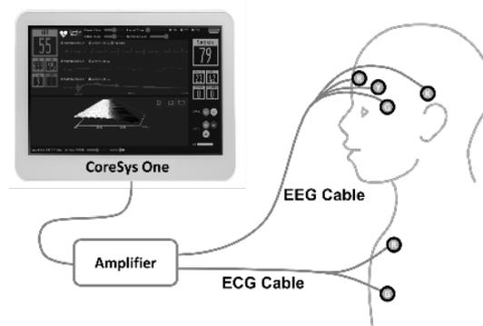
Figure 1 CoreSys One monitor with the position of the EEG/ ECG electrodes.
